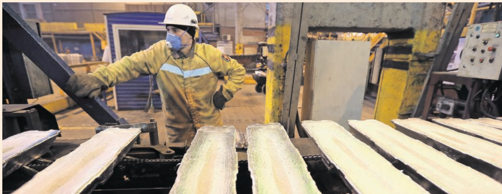
A worker watches as aluminum ingots pass along a conveyor belt after cooling in the foundry at Rusal's smelter in Krasnoyarsk — Andrey Rudakov/Bloomberg
